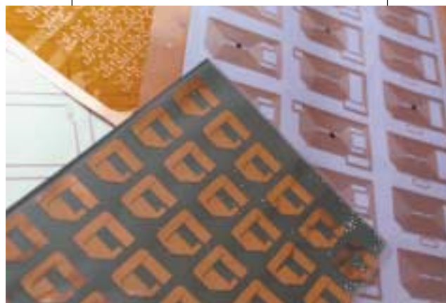
This is an example of a typical flexible printed antenna for wireless applications.
